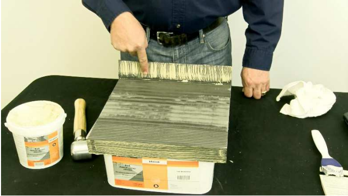
Give the adhesive a light touch. When there is no transfer to the fingers, the adhesive is ready. You have two hours of working time, once the adhesive reaches the dry to the touch state.
